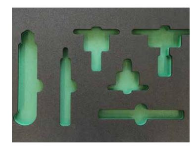
Not only is it essential to protect tools in storage, it is equally important to have a means of controlling their use. Looking for the right tool in a drawer full of tools or having to go searching for a missing tool can result in the loss of valuable production time. The solution is a two-tone foam insert. If the toolkit changes it is also easy to modify the program.
